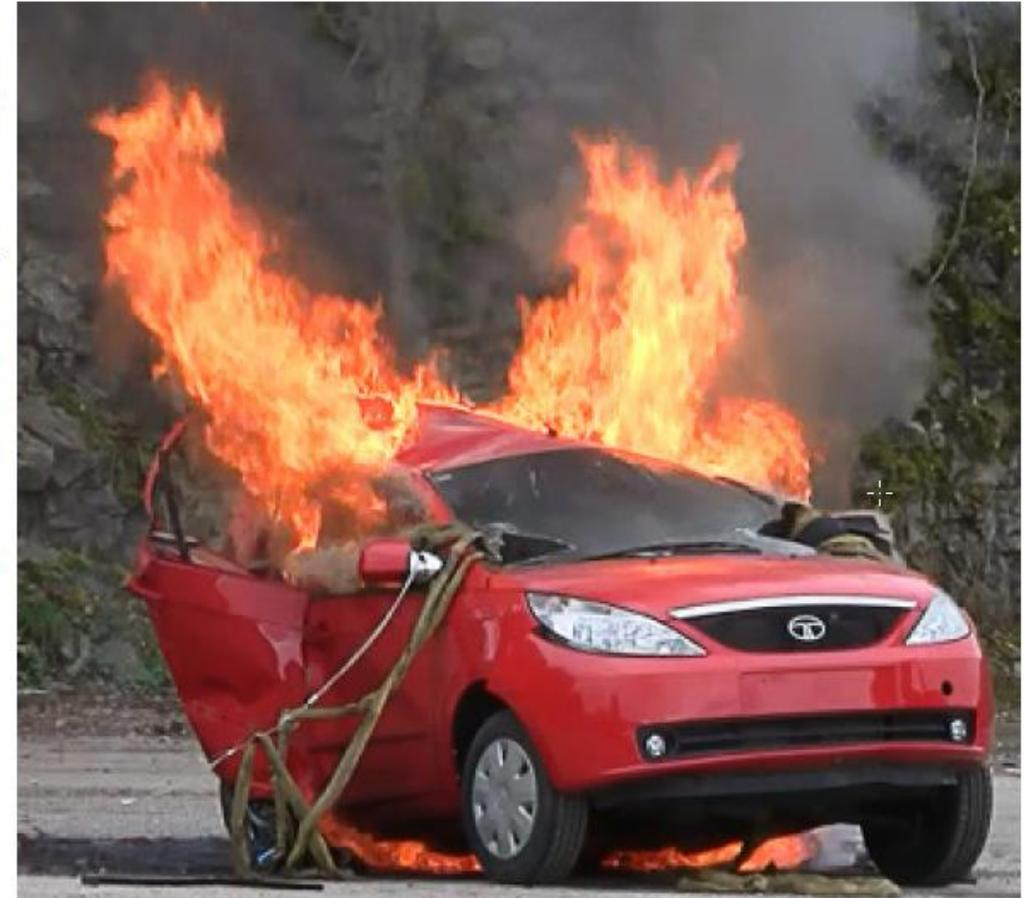
**Figure 5 Test 1 – The photo is taken 8 minutes after the drop. At this point the car has started to burn vigorously.**
