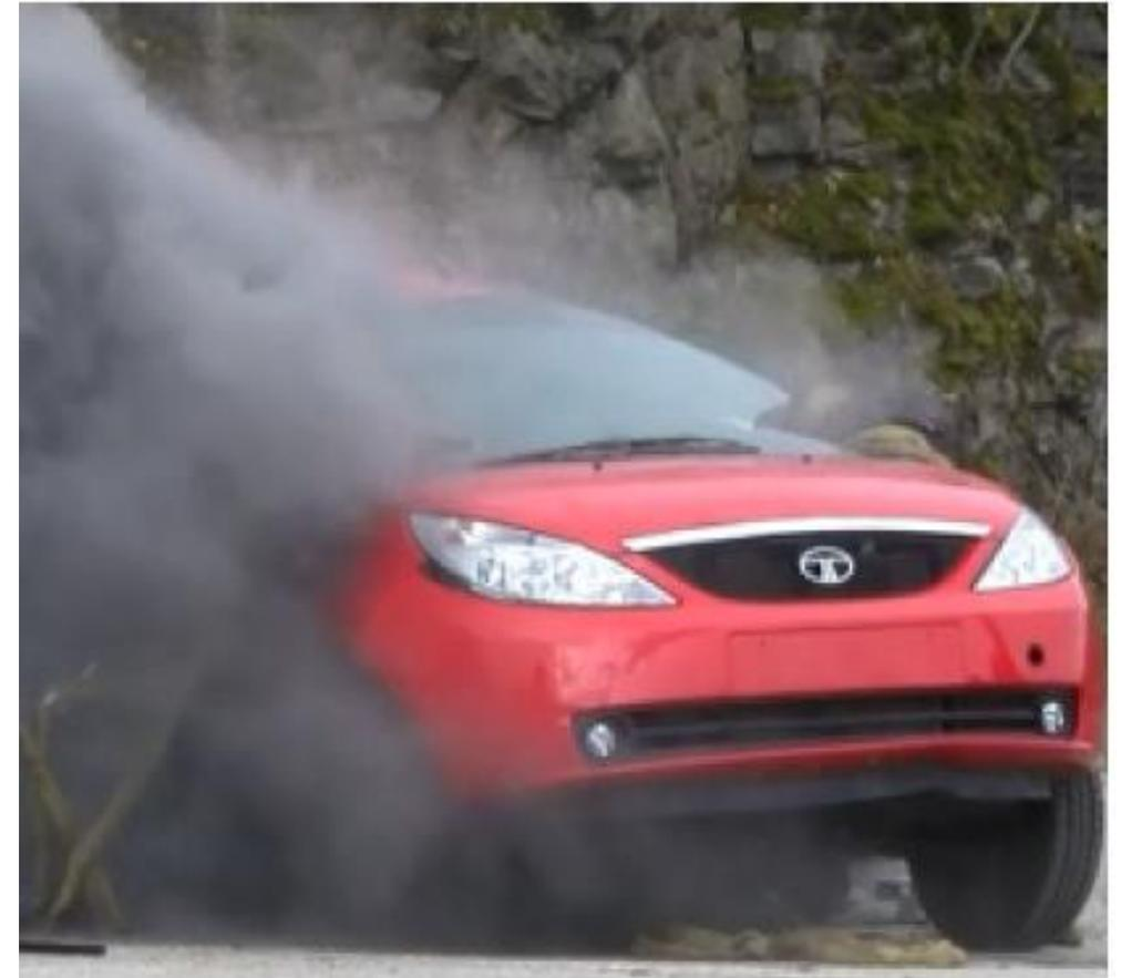
**Figure 4 Test 1 – The photo is taken 2 min after the drop, and large amount of smoke are produced from the battery**
