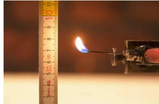
The IEC TS 62441 needle flame
