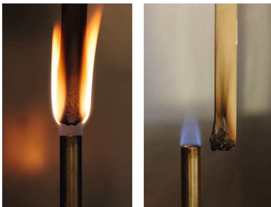
Fig. 1. Core question for the ENFIRO project: How good in reality are the non-halogenated flame retardants in plastics – during the fire test (left) and after passing the test (right) (photos: Clariant)
