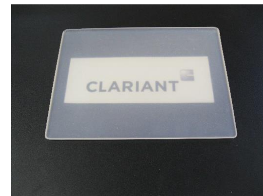
Epoxy sample containing ATH, 40 phr
