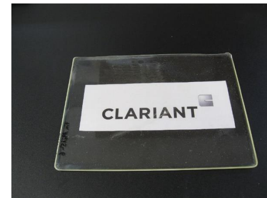
Epoxy sample containing Exolit EP 360, 3 wt% P
