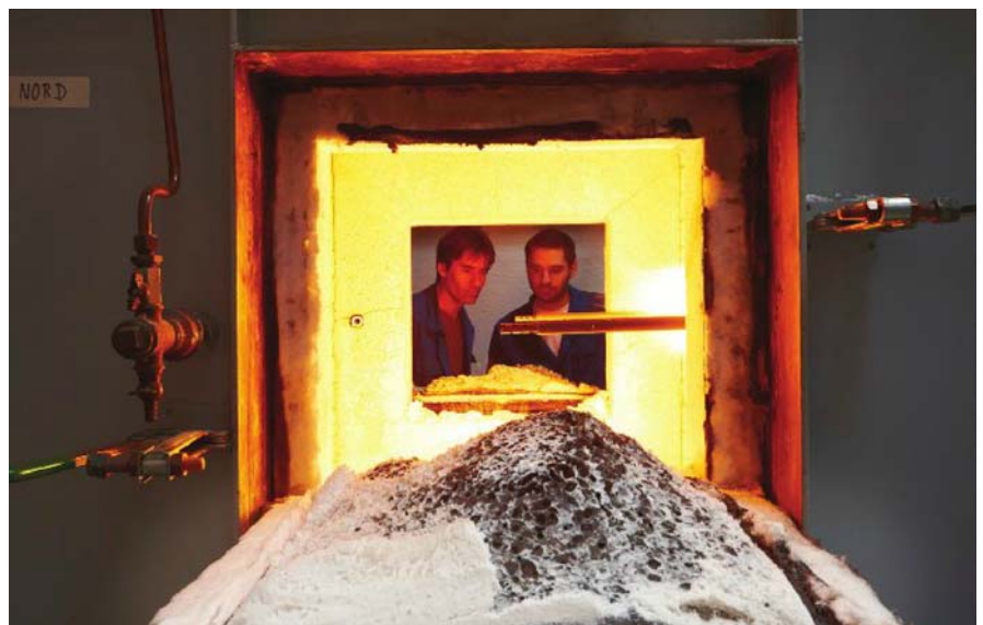
View through a test furnace at the German Federal Institute for Materials Research and Testing showing the intumescent coating sample after test
