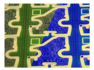
"To be blue or not to be blue, that's the question ..." Shakespeare would have posed: Currently, green is the common colour of printed wiring boards containing brominated flame retardants, whereas blue is used for materials with non-halogenated flame retardants.
